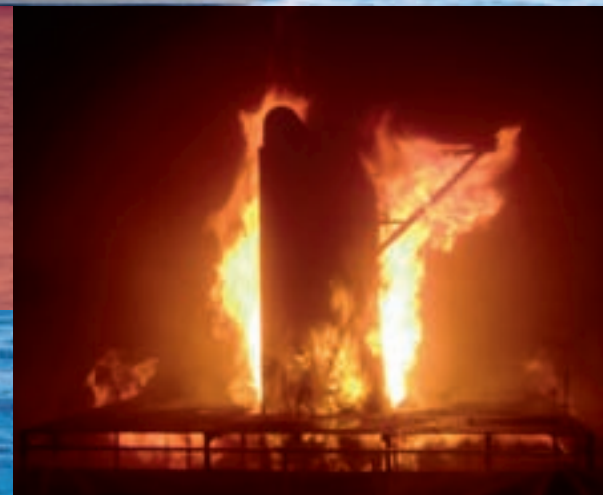
Machinery spaces (bilge) test according to IMO-MS/Circ. 1165
